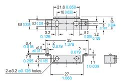
Material: Cold rolled carbon steel (SPCC) (Uni-chrome plated)
