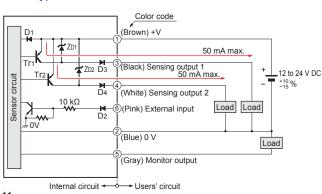
Non-voltage contact or PNP open-collector transistor
