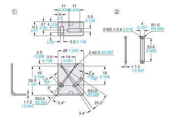
MS-EXL2-1 Sensor head mounting bracket for **LS-H102**□ (Optional)
