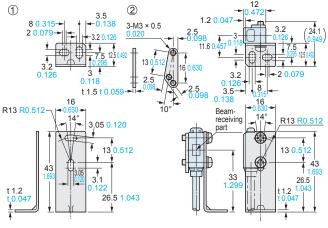
Material: Stainless steel (SUS304) Two M3 (length 14 mm 0.551 in) screws with washers [stainless steel (SUS304)] are attached.
