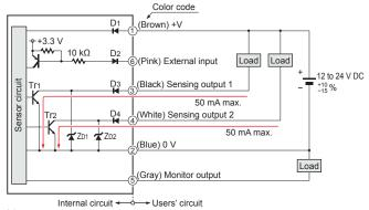
Non-voltage contact or NPN open-collector transistor
