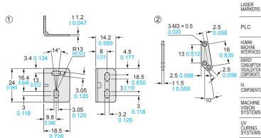
Material: Stainless steel (SUS304) Two M3 (length 14 mm 0.551 in) screws with washers [stainless steel (SUS304)] are attached.
