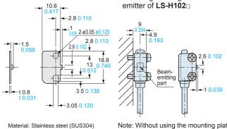
Note: Without using the mounting plate, beam misalignment may occur.
